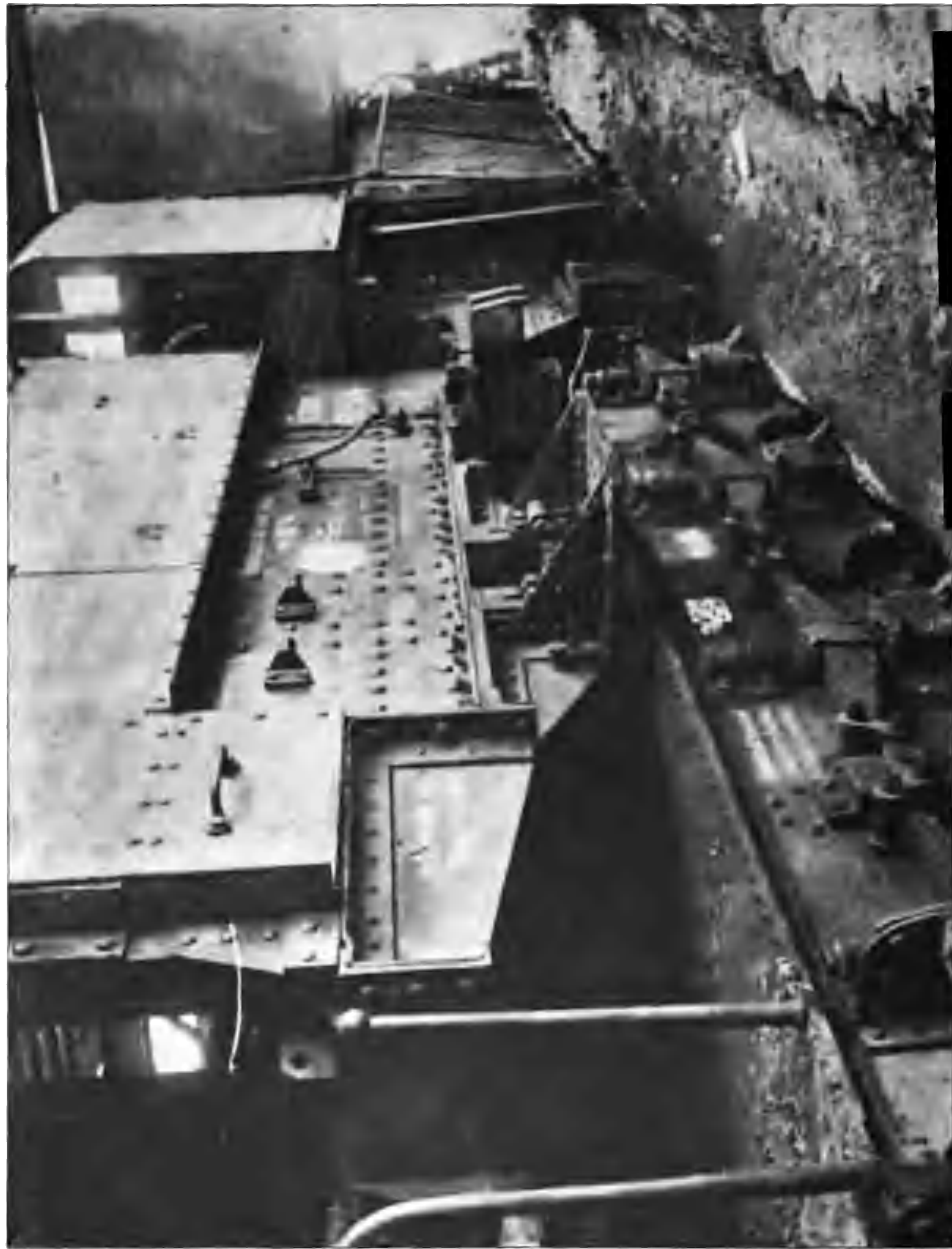
TRUCK TRAVERSING MECHANISM AND JACKING BEAM OF THE 240-MM. GERMAN HOWITZER MOUNT.
