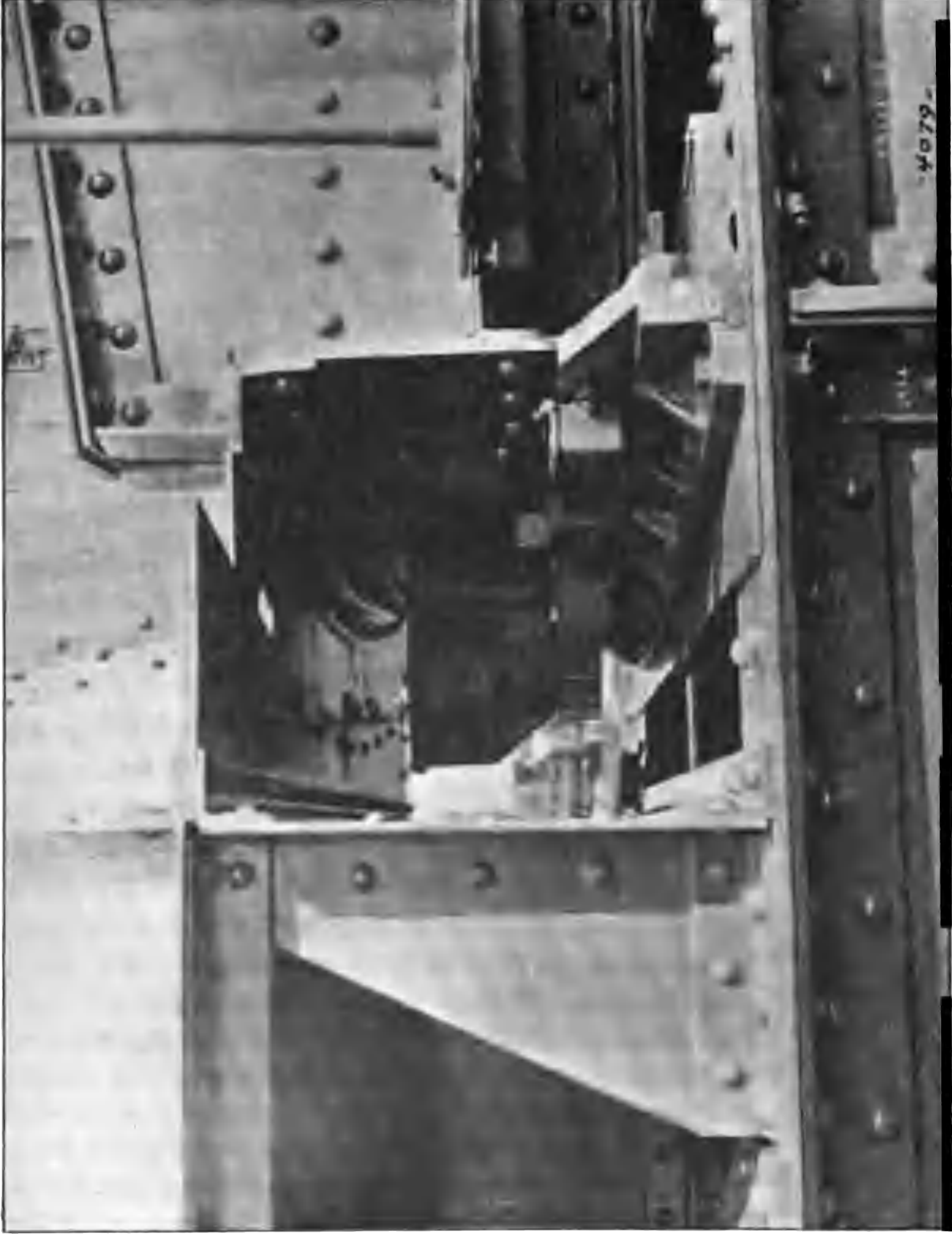
RACK AND PINION OF THE TRAVERSING MECHANISM OF THE 12-INCH, 35-CALIBER AMERICAN GUN MOUNT.
