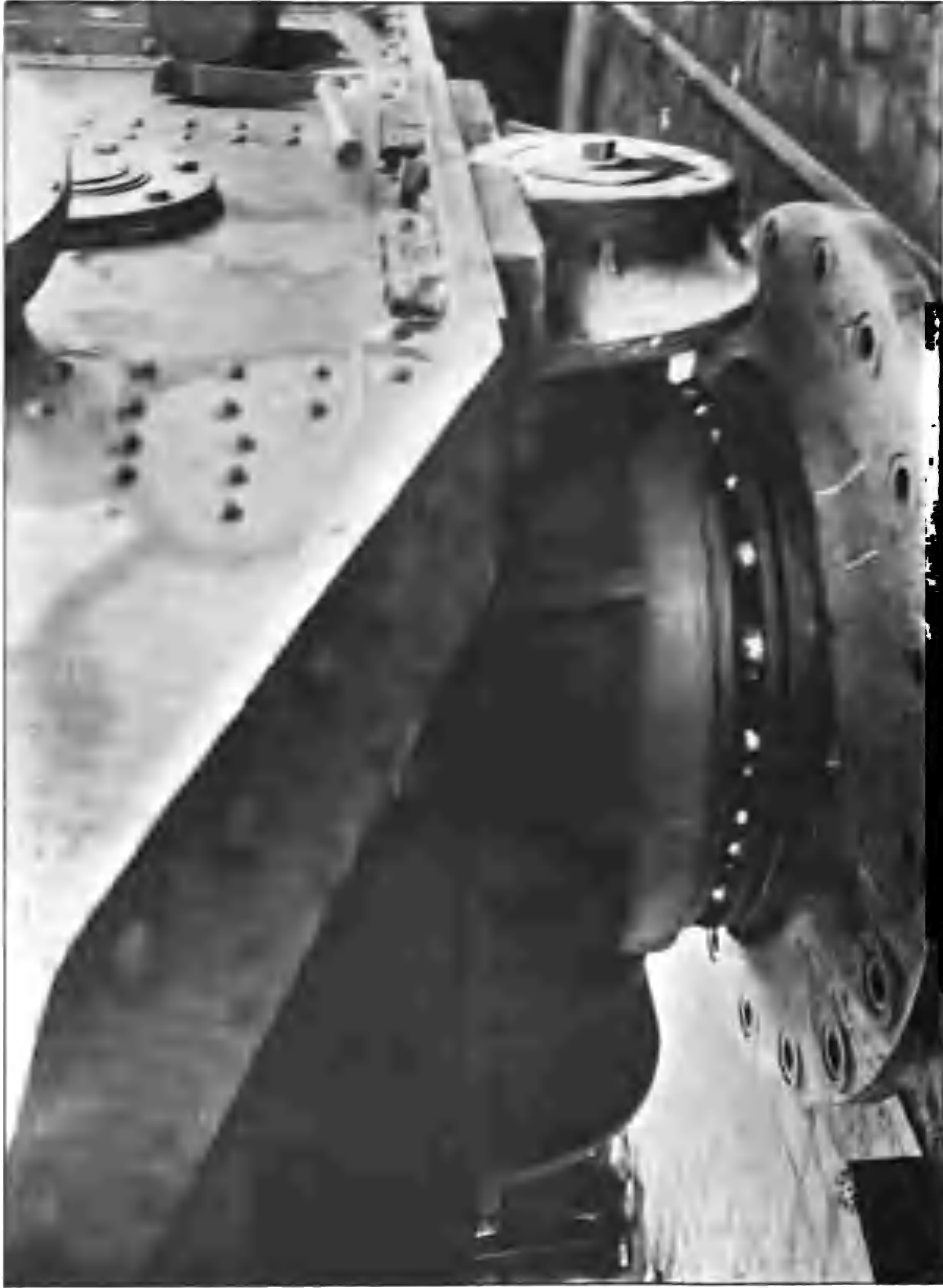
CENTER PIVOT OF THE 280-MM. GERMAN GUN MOUNT.
