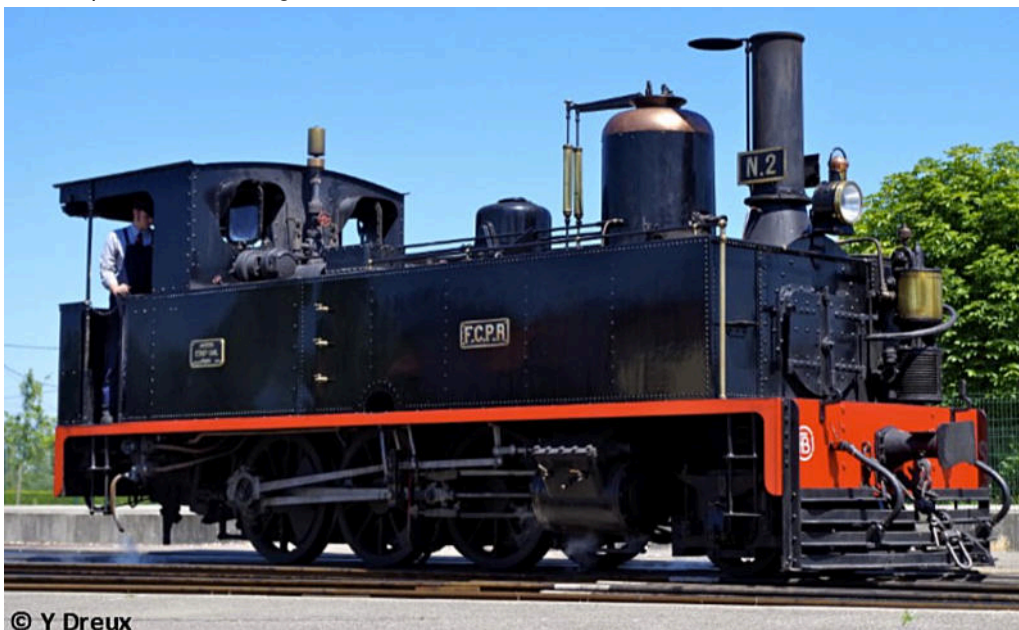
No. 2 as it is nowadays, back in France and running at the Chemin de Fer de la Baie de Somme . An air-pump and turbo-generator have been added, when compared with the image above.
