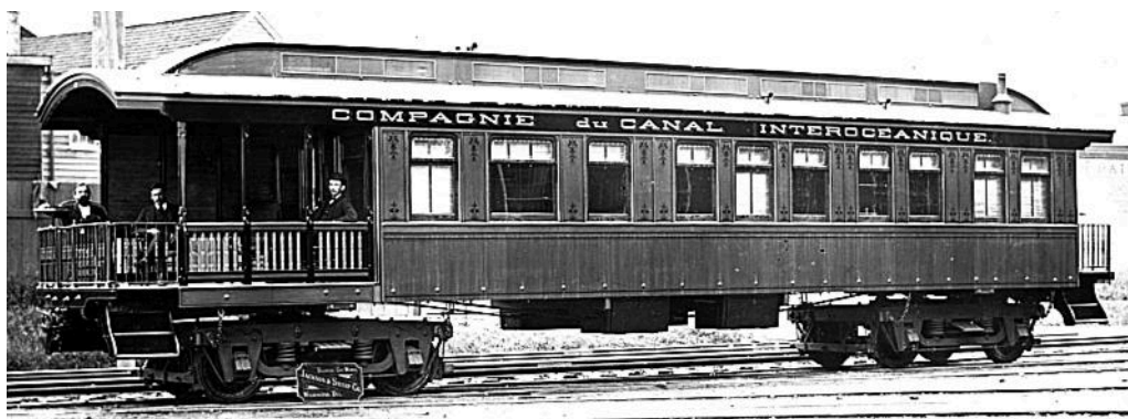
A CUCI car built by Jackson & Sharp in Delaware, before shipment to the isthmus. Presumably this was an officers' inspection saloon of some kind, as the compagnie did not run passenger services as such.
