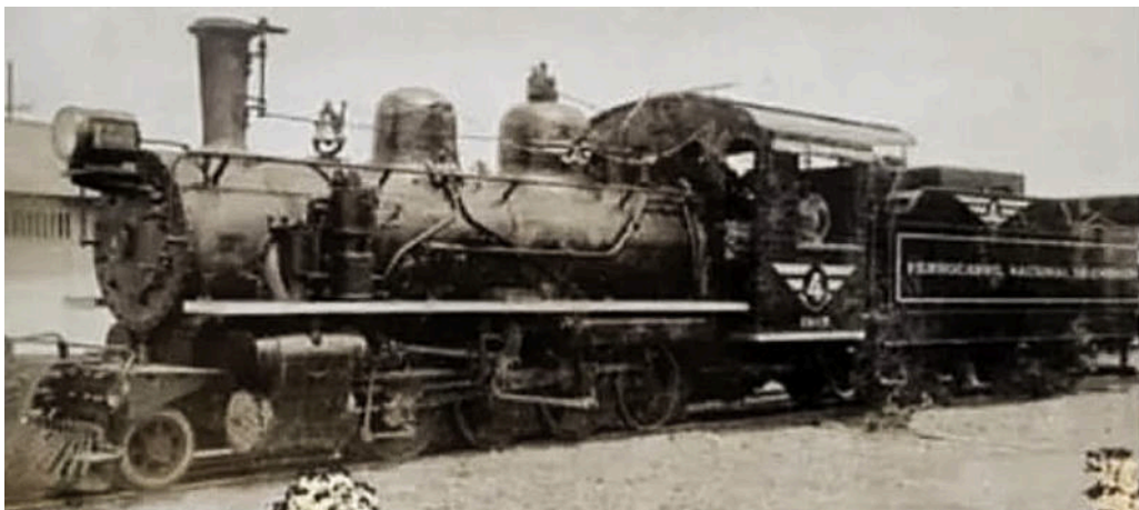
No. 4 was clearly an updated ALCo version of no. 3, with piston valves instead
