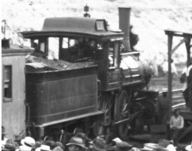
Another cropped enlargement from a view of the pay train. Charles Small [15] said that this was Cooke 4-4-0 no. 57 . Certainly the single tender rivet line just below mid-height, and the matching height of the bottom of the cab, recall the Cooke locos rather than the zigzag rivet line of the Baldwins.
