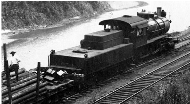
No. 654 on a train, showing the flat-topped tender tank, with a relatively small bunker totally filled by the oil fuel tank.
