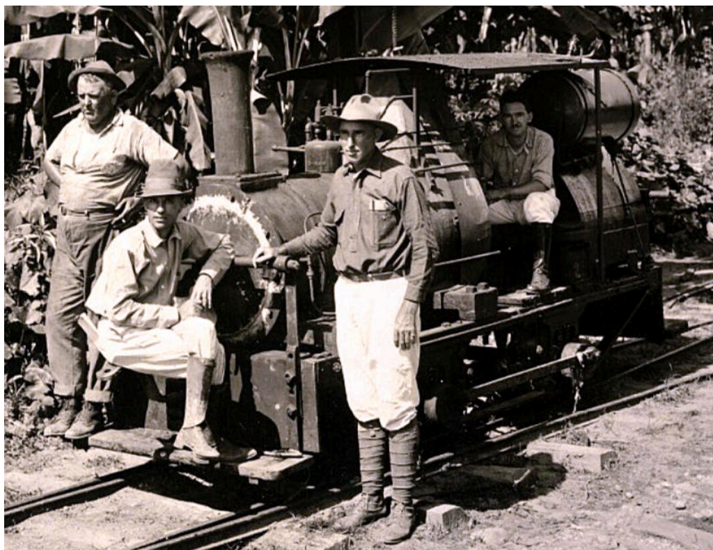
A UFCo photo showing a Bell geared loco, presumably on one of the company's rail systems.
