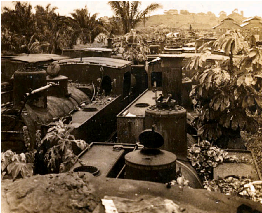
Derelict French locos at Empire, as seen in a stereoscopic lantern slide. The engine in the foreground and that to the left are of the larger type, F-B type 27, whilst that a little further ahead from the camera is one of the smaller class (F-B type 88).
